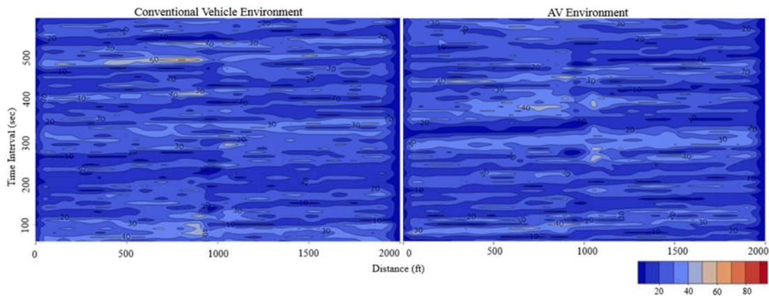
Figure 3. Vehicle Density for Lane One under LOS B.
