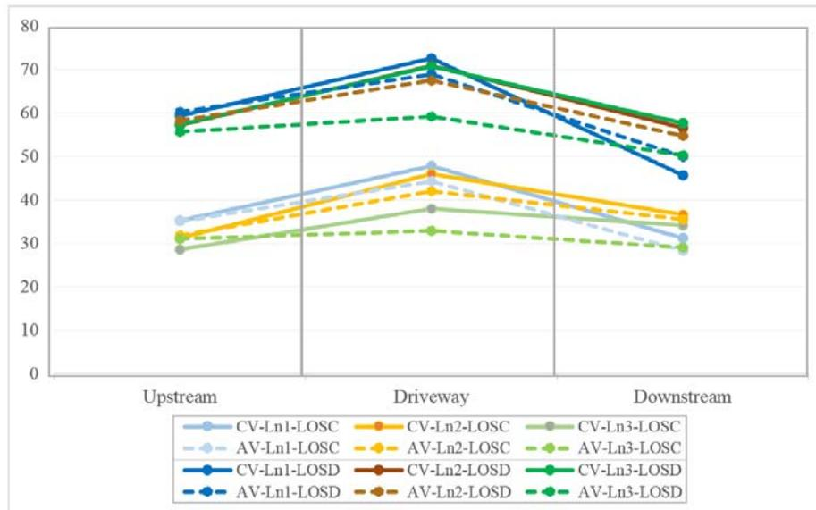
Figure 6. Percent of the Times with Traffic Blockage under LOS C and LOS D for in the Conventional Vehicle Environment vs. AV Environment.
