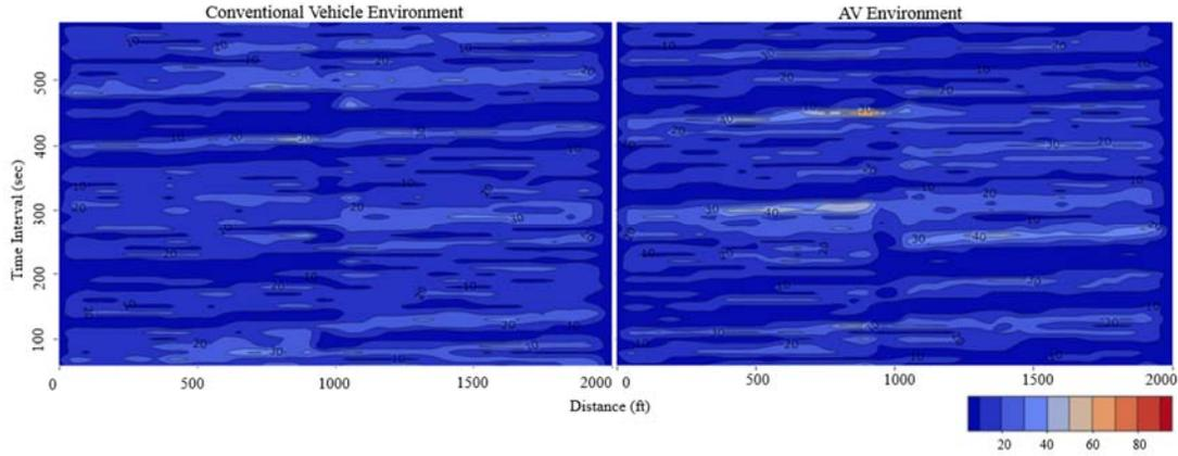
Figure 2. Vehicle Density for Lane One under LOS A.
